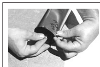
Peg firmly with the bolt and nut provided, and slide your pipe onto stove surface (next page)
